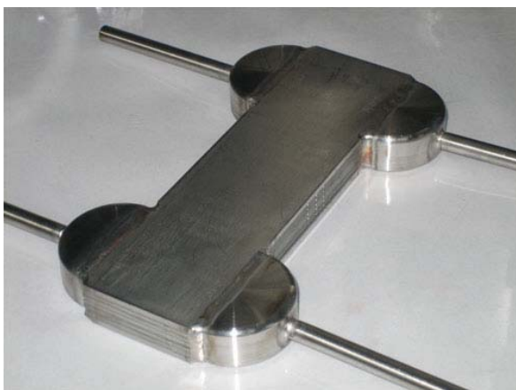
Fig. 3 The microchannel PCHE using the diffusion bonding technology
