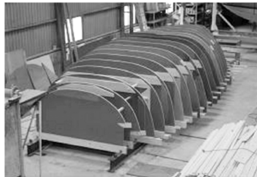
Fig. 5. Frame arrangement of hull mould.
