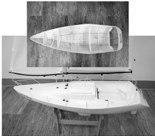
Fig. 2. Rapid prototyping model of design ship.
