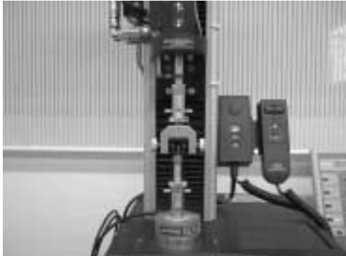
Fig. 5. Test assembly attached to tensile testing machine and tensile test
