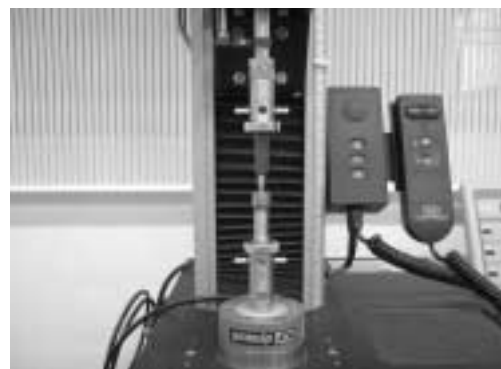
Fig. 4. Cementation using Instron Universal Testing Machine
