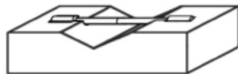
Fig. 1. Stone block for laser welding
