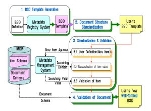
(Figure 3) Concept framework of BSD Creator
