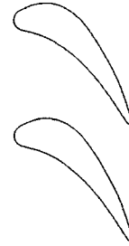
Fig. 2 The shape of calculated turbine nozzle
