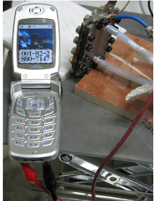
Fig. 10 Demonstration of the cellular phone powered by 6 cell stack PEMFC
