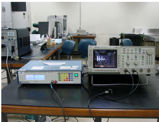
Fig. 3 Ultrasonic propagation property measurement system
