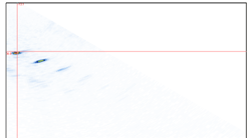
Fig. 15 Sectorial signal from 60-70 mm SDH
