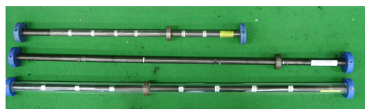
Fig. 4 Calibration standard & flaw specimen for magnetic saturation ECT
