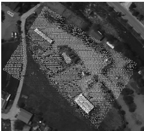
Fig. 6. Back-projected LiDAR points overlaid with one of stereo images
