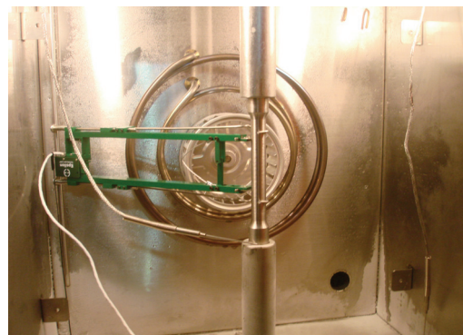
Fig. 5 A photograph of Extension meter installation in a cryogenic chamber
