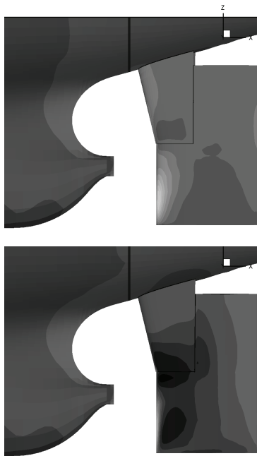
Fig. 12 Pressure contour at -10 degrees (Upper : Stb. Side, Lower : Port side)
