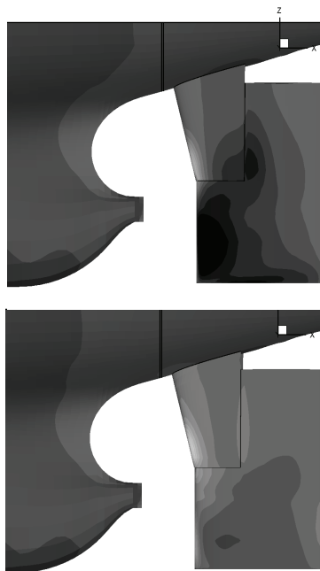
Fig. 12 Pressure contour at -10 degrees (Upper : Stb. Side, Lower : Port side)
