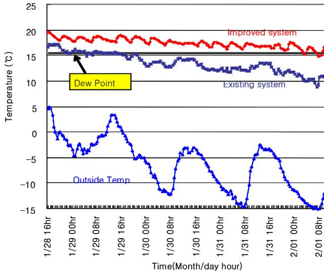
Figure 14. Surface temperature distribution of door frame
