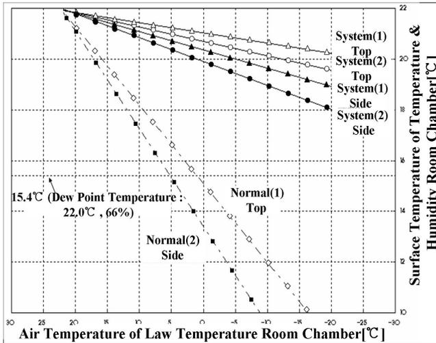
Figure 11. Surface temperature of door frame by mock-up test
