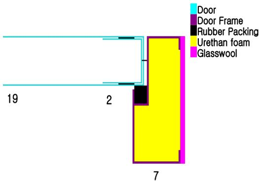
Figure 6. Adhesive tape design of door
