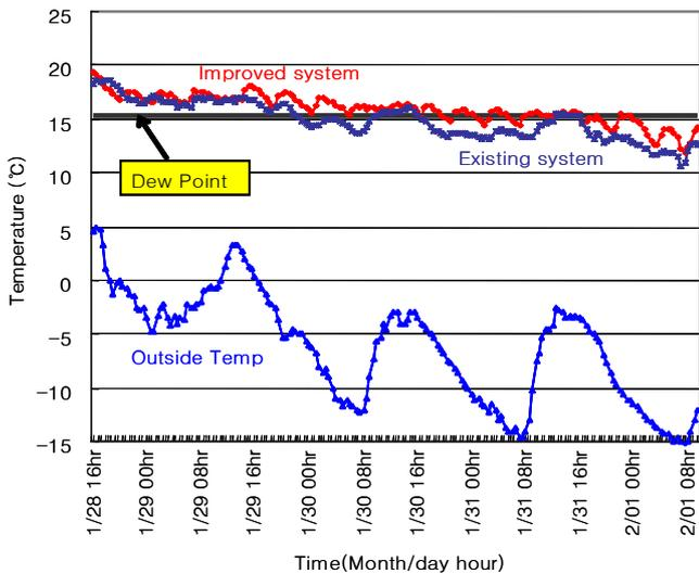
Figure 15. Surface temperature distribution of door
