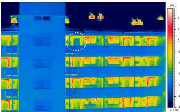
Figure 16. Temperature distribution of units by infrared ray camera
