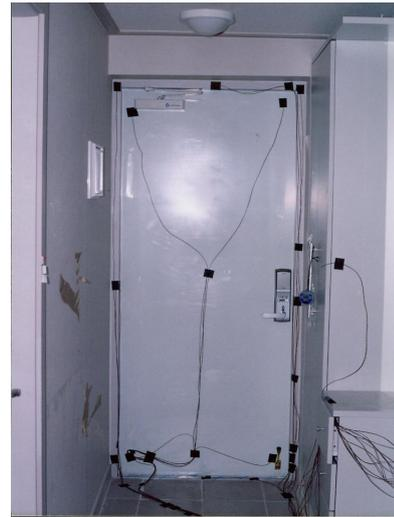
Figure 13. Measurement point of surface temperature
