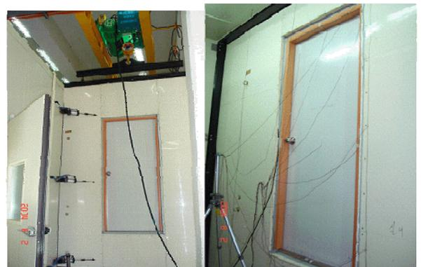
Figure 10. Specimens for condensation test
