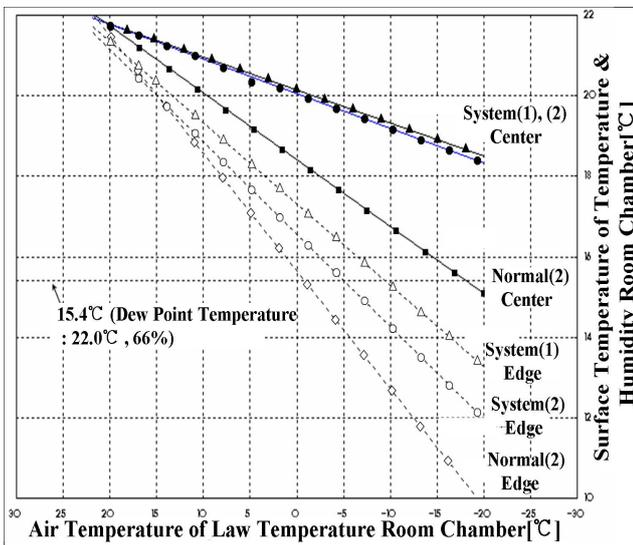
Figure 12. Surface temperature of door by mock-up test
