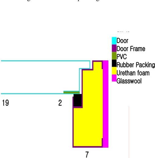
Figure 7. Bent frame design of door
