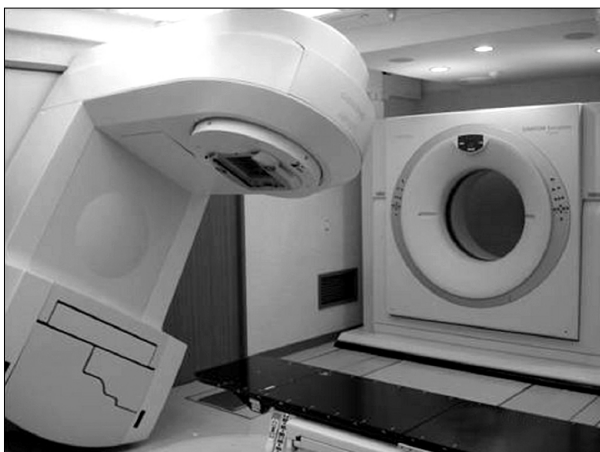
Fig. 1. The image of CT on-rail system. It consist of LINAC (ARTISTE, Siemens) and CT scanner (Sensation open, Siemens).
