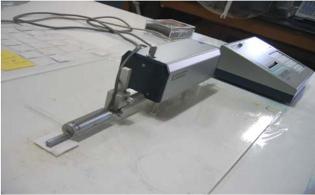
Fig. 1. Photograph of surface roughness measuring instrument (Surfcoorder SE1200).
