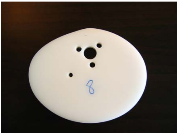
Fig. 10 cam3 made of polyacetal (2,3)
