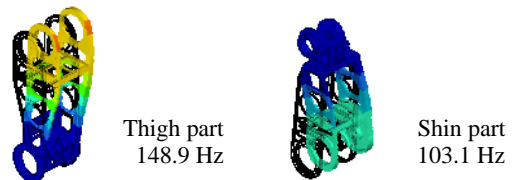
Fig. 8 Stress contour and graph of the lower parts
