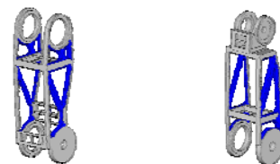
Fig. 9 The results of the lower parts for topology optimization
