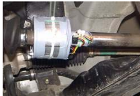
Fig. 4 Strain gages and telemetry system
