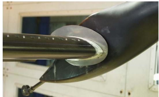
Fig. 3 The installed wingtip fence on model
