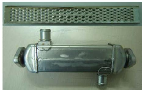
Fig. 2 Dimpled rectangular tube EGR Cooler
