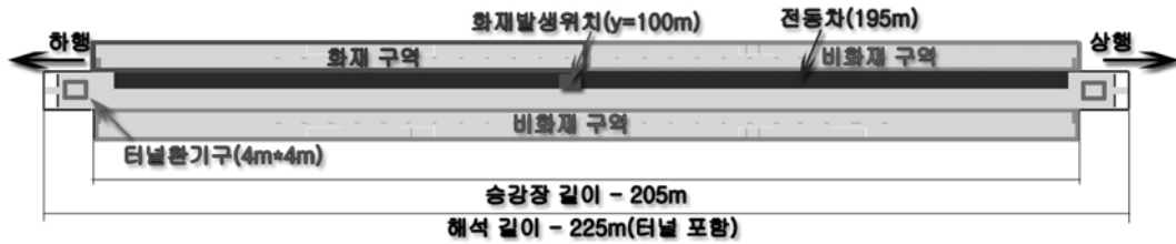
Fig 3. Zones and fire location on the platform
