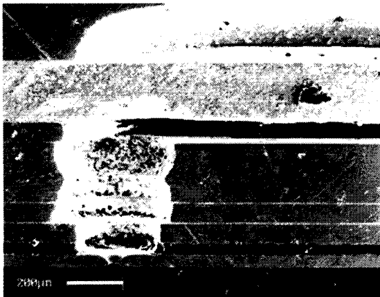
Fig. 4 Imperfections of a piezo Drop-On-Demand inkjet print head in the 90's by Spectra, Co. 17
