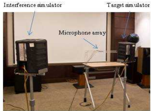
Fig. 4 The experimental setup
