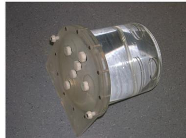
Fig. 1. Phantom (Uniform NU2-94 Phantom).
