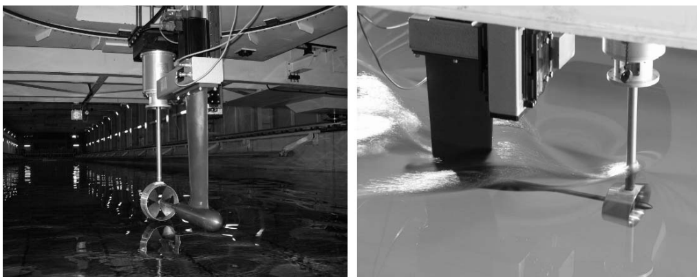
Fig. 5. Experimental scene by propeller open water (POW) tests.
