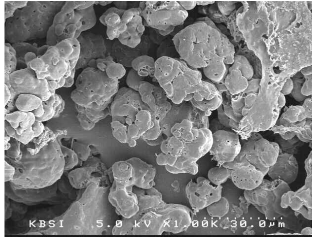
Fig. 2. Field emission scanning electron microscope micrograph of the three-layer coated Bacillus polyfermenticus KJS-2.
