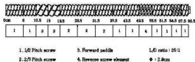
Fig. 1. Screw configuration for ginseng process (model THK 31T).
