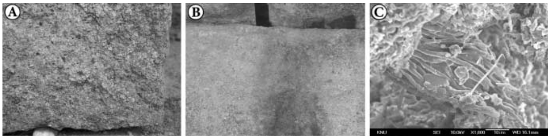
Figure 9. Representative biological weathering of host rocks for the stone Buddhas and Shrine. (A) Green foliose covers the wall rock. (B) Surface green discoloration by green algae. (C) Scanning electron microscope image of organic rootlets grown into the host rock.
