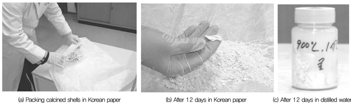
Figure 7. Slaking of calcined shells.
