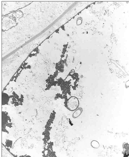
Figure 7. Transmission electron micrographs for cross section of Alnus spp. (×4,400), Degradation of vessel cell wall by soft rot.
