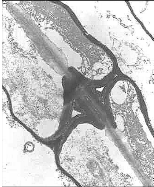
Figure 5. Transmission electron micrographs for cross section of Alnus spp. (×12,000), high decay-resistance of S3 and pit membrane, and extensive degradation of S2 wall.
