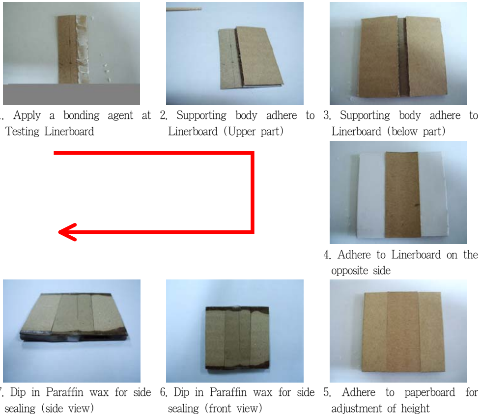
Fig. 3. Preparative Process of Test Specimen
