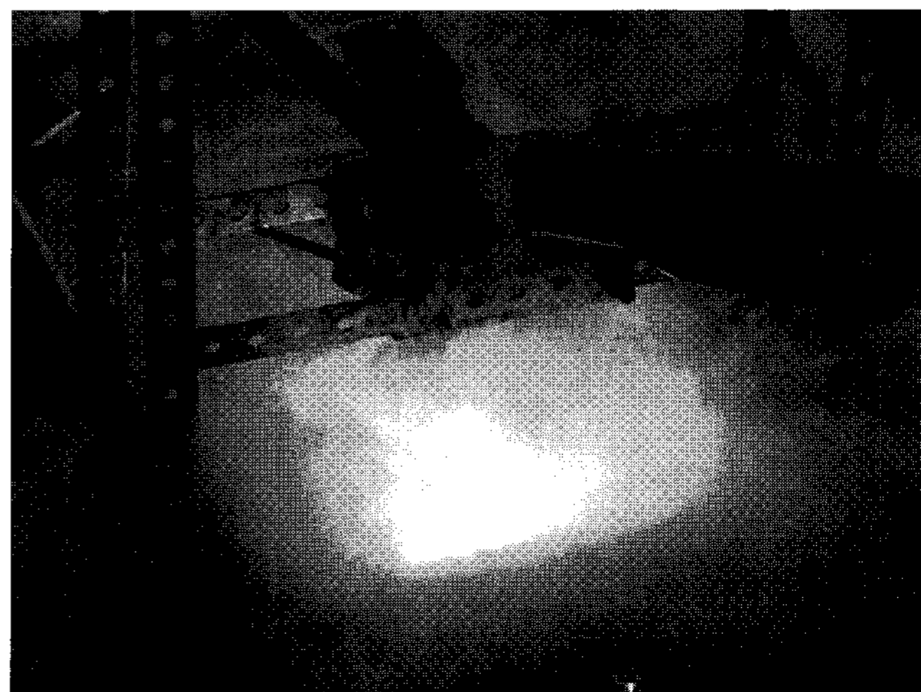
Fig. 1 Graphite cathode and anode arc-discharge in liquid nitrogen in the experiment
