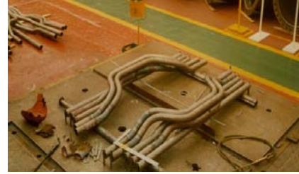
(a) Assemble work of the short tube pieces.
