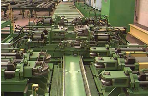
Fig. 8 Overview of the developed 3D bending machine
