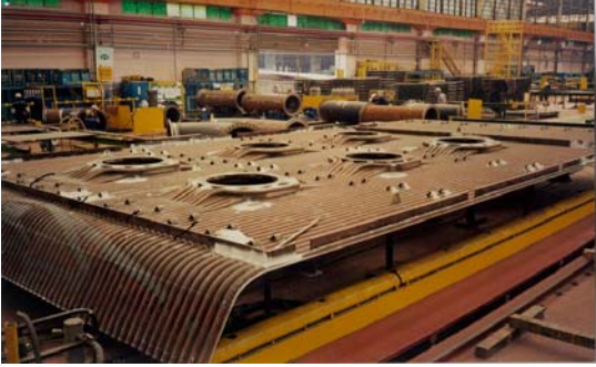
Fig. 1 Appearance of the boiler panel
