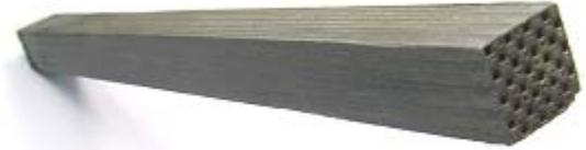
**Fig. 1** Configuration of modified CDPF for rig test
