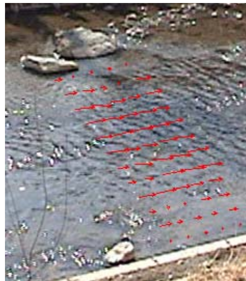
Fig. 5. Velocity field measured with SIV
