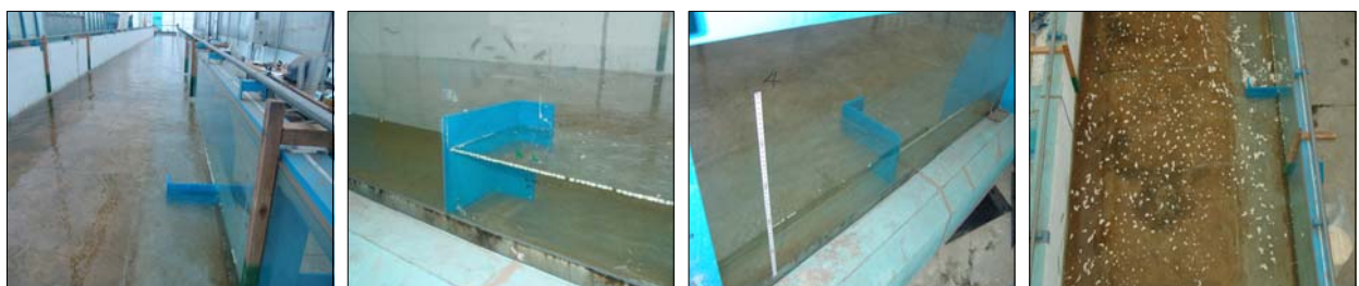
Fig. 6. Experimental Setting on L-type Groyne
