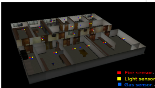
Fig. 8. 3D Responsive Virtual URS – 3D visualization of sensor distribution
