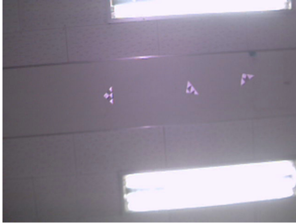
Fig. 5-(a). Landmarks with IR LED ON
