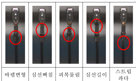
Fig. 10. The bad sample of wire harness.
