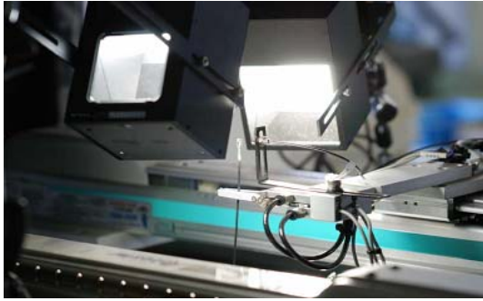
Fig. 12. The inspection apparatus of wire harness.
