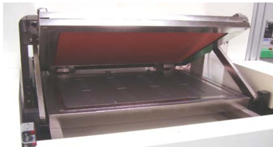
Fig. 10. Vacuum Attached Chamber of Movable Pocket.
