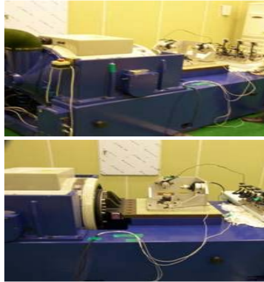
Fig. 12. Equipment of vibration test.
