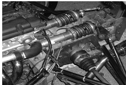
Fig. 4. Rear suspension of F 1800 race car.
