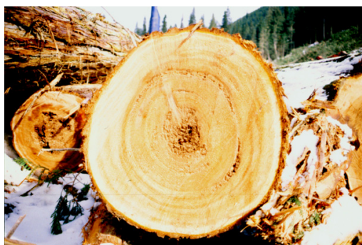
Fig. 4. Pocket and ring rot in western red cedar.
