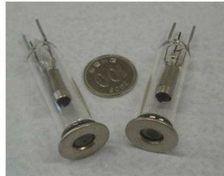
FIG 2 Picture of the developed x-ray transmission tube
