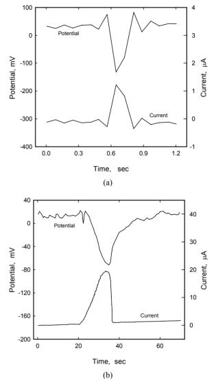
Fig. 2. Typical transients observed after 74 hours(a) and 144 hours(b) of exposure to 3.5% NaCl solution.
