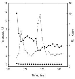
**Fig. 5.** Kurtosis of current( $\bigtriangledown$ ), localization index(( $\bigcirc$ ) and noise resistance( $\square$ ) as a function of time for the data in Fig. 4.
