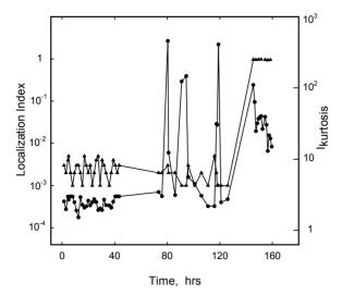
Fig. 1. Plot of Localization index( $\blacktriangle$ ) and kurtosis of current( $\bigcirc$ ) as a function of exposure time.
