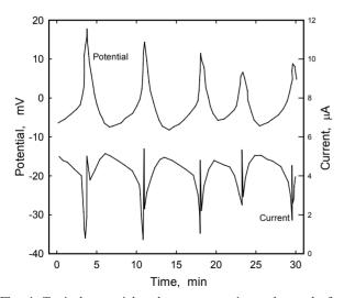
Fig. 4. Typical potential and current transients observed after exposure to 3.5% NaCl solution for 7 days.
