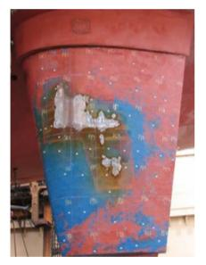
Fig. 2. Typical cavitation induced corrosion damage of ship's rudder  $^{\rm l}$
