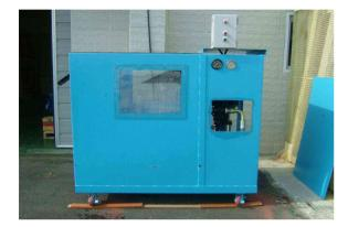
Fig. 4. Water-jet cavitation erosion tester
