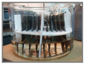
Fig. 5. Immersion test in sulfuric acid of fluoroelastomers(95%  $\rm H_2SO_4,~90\,^\circ\!C)$
