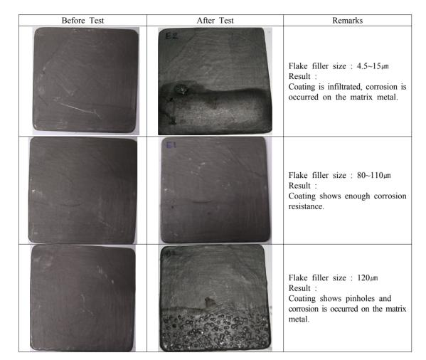
Fig. 6. Immersion test result in sulfuric acid of coating with various flake filler size
