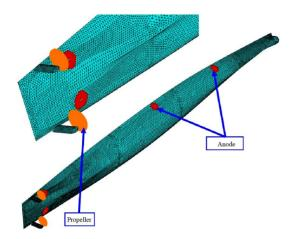
Fig. 2. Boundary element model of ship hull including propellers and rudders(Six anodes double zone ICCP system, 2% coatings loss)
