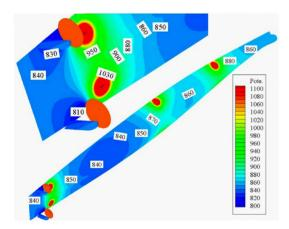
Fig. 3. Potential contours on the ship hull including propellers and rudders (mV.Ag/AgCl)(Six anodes double zone ICCP system, 2% coatings loss)
