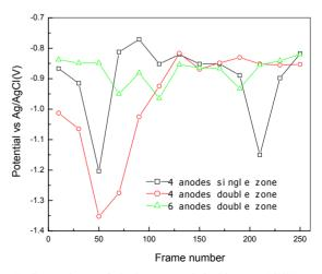
Fig. 5. Comparisons of single zone and double zone ICCP system of model ship
