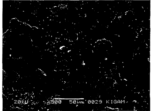
Fig. 5. SEM image of heat treated sample at 1050^\circ\text{C} .
