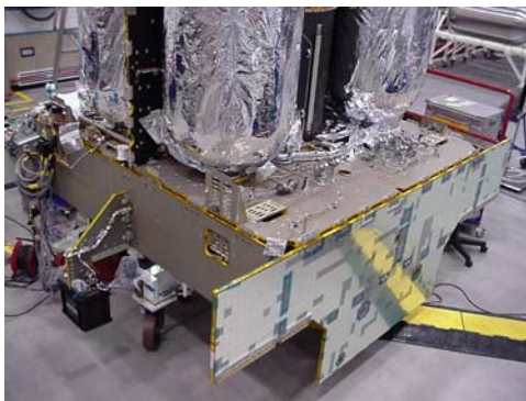
Fig. 5 Eurostar 2000 Chemical Propulsion System Manufactured in Stevenage, UK
