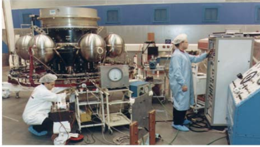
Fig. 6 CPS Functional Test
